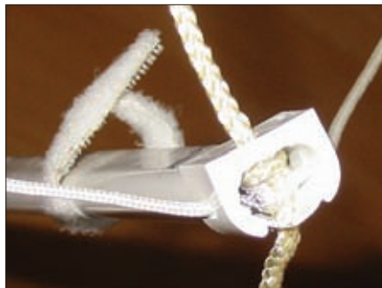
Fig. 2: The tensioning (thicker) and circumferential (thinner) cords are located in the end of the oval conduit using 'figure of eight' stopper knots. One of the Velcro tapes for attaching the dish panels is also visible.
