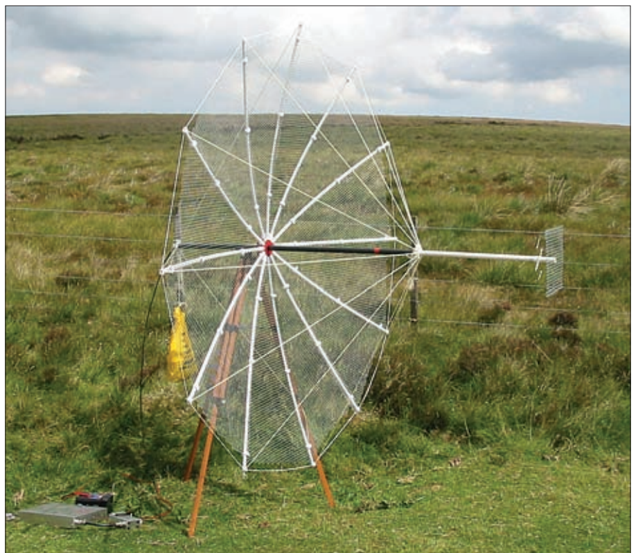
Fig. 8: The counterweight mounted on the end of the support pole; the four rear tension cords are visible.
