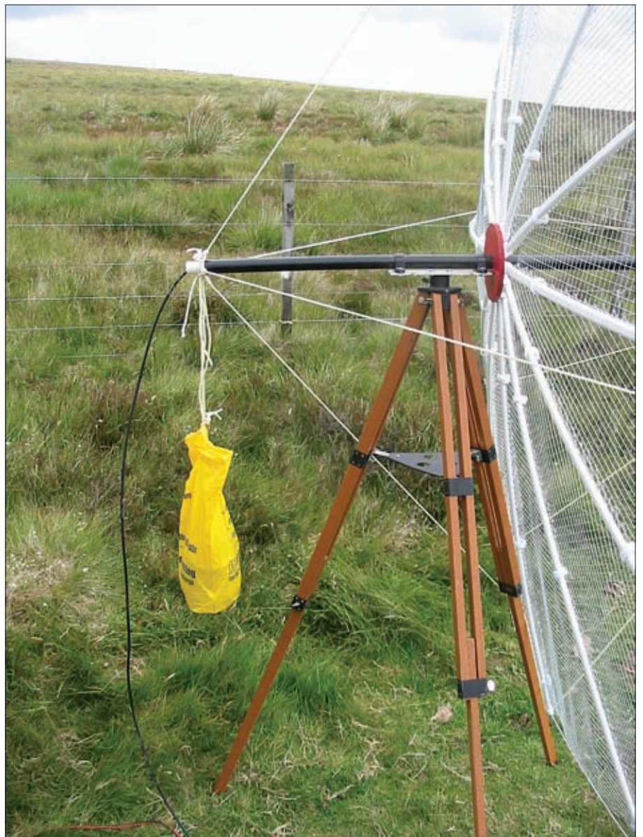
Fig. 8: The counterweight mounted on the end of the support pole; the four rear tension cords are visible.
